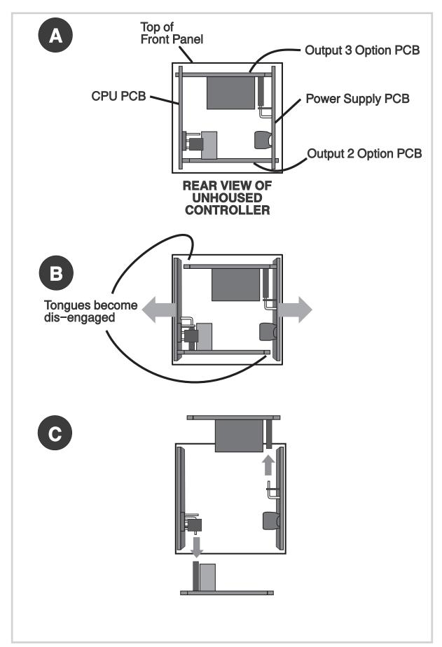
Figure 2-2 Removing the Output 2/Output 3 Option PCBs
